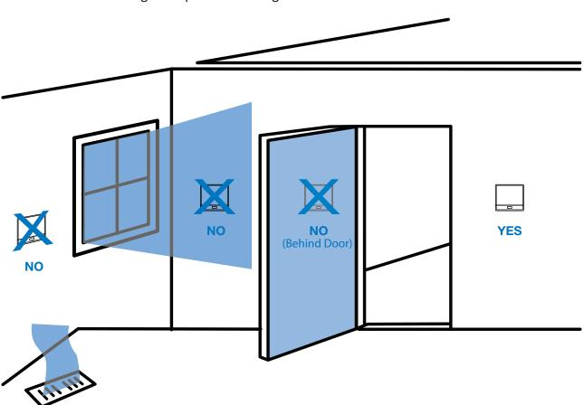
The thermostat should be installed approximately 4 to 5 feet above the floor. Select an area with average temperature and good air circulation.
